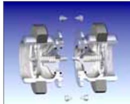
When the safety break-away couplings are separate, it allows the two poppets to close. The two poppets close rapidly, minimizing exposure to personnel and the environment.
